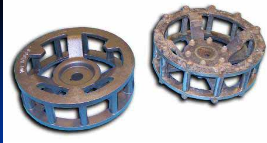
Ductile Iron Drive Wheel Converted From Fab
